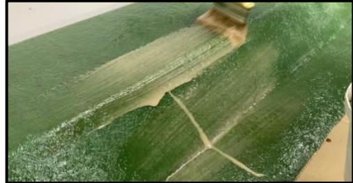
*Add a coat of PO80 prior to the keyed surface prior to adding the first 450g CSM*
