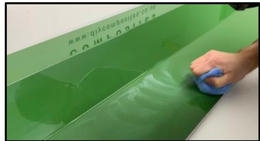
We recommend using our preferred PAI Just 1 polish for gel coat surfaces such as this. The polish acts not only as cutting compound but also a polishing compound to help give an excellent final shine. This can easily be completed with a polishing wheel or by hand with a simple 2 cloth (microfibre) approach. One cloth to put on and polish in circular motions and another cloth to buff off.
